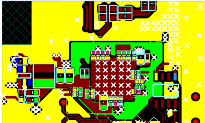
Figure 4.11: 2.5V Plane (Green Plane) of Bottom Layer.
