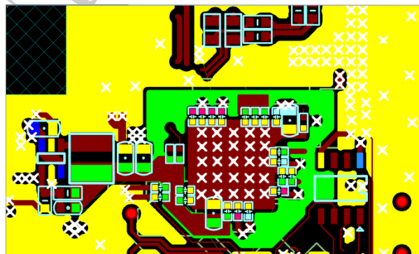
Figure 3.8: 2.5V Plane (Green Plane) of Bottom Layer.
